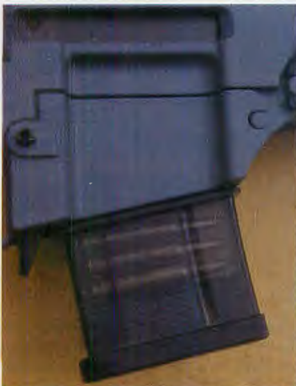
Using a special magazine well, the SL8-1 will accept only its unique 10-shot in-line magazine.
